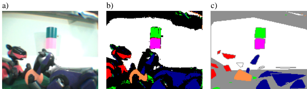
Figure 3.1: From an image to blobs. a) The original image, b) The segmented image, c) The detected blobs.
