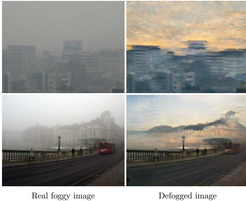
Figure 4.3: Some example of poor defogging, where some elements of the image are transformed in clouds and blended into the background.
