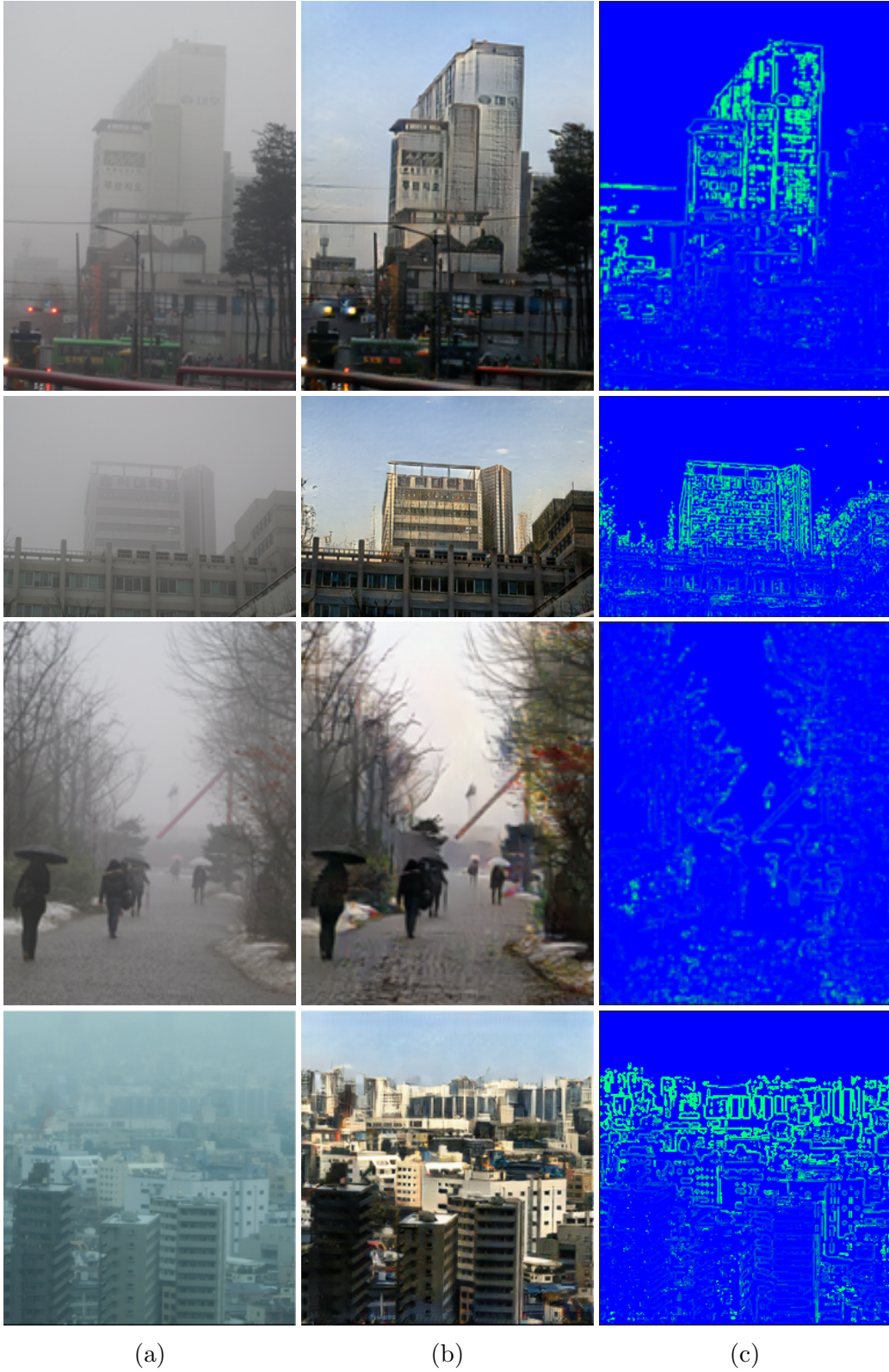
Figure 4.8: Some example of defogging using the unpaired approach adopted in this dissertation II. (a) real hazy image (b) the resulting defogged image (c) contrast enhancement map.
